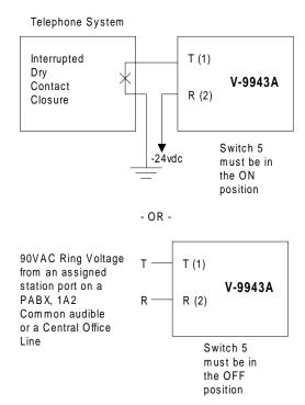
The V-9943A is activated by 70-105 Vac (ring voltage) or -24 Vdc (normally through an interrupted contact closure). If the V-9943A is to be connected to the telephone network, two wires should be secured to the screw terminal connection on the PCB. The other end of the wires should terminate at a RJ11C jack.
